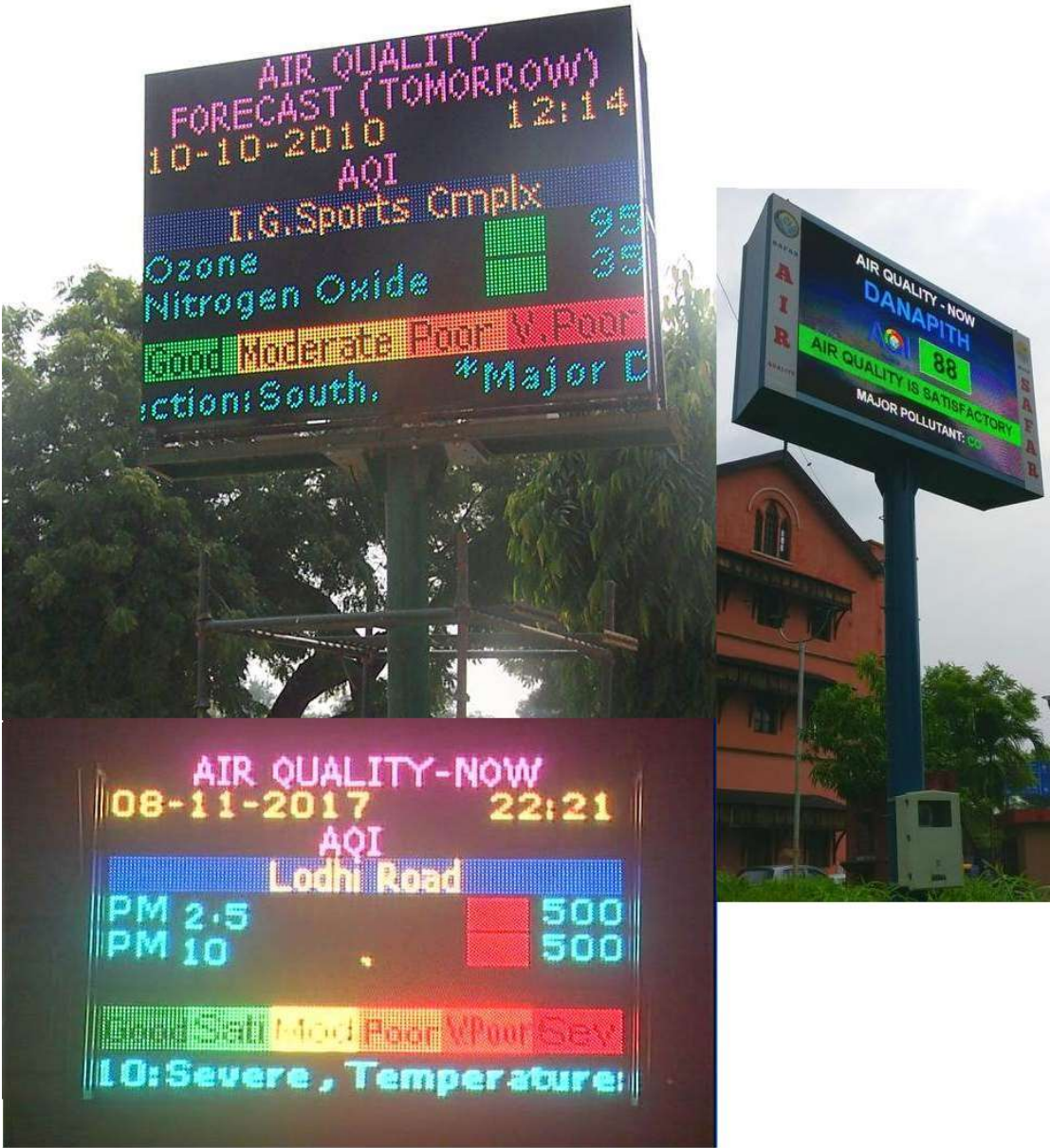
Figure 20 : Variable Message Board displaying values of Particulate Matter PM2.5 and PM10 and Current value of Air Quality Index along with Color Code and Value understood by citizens
