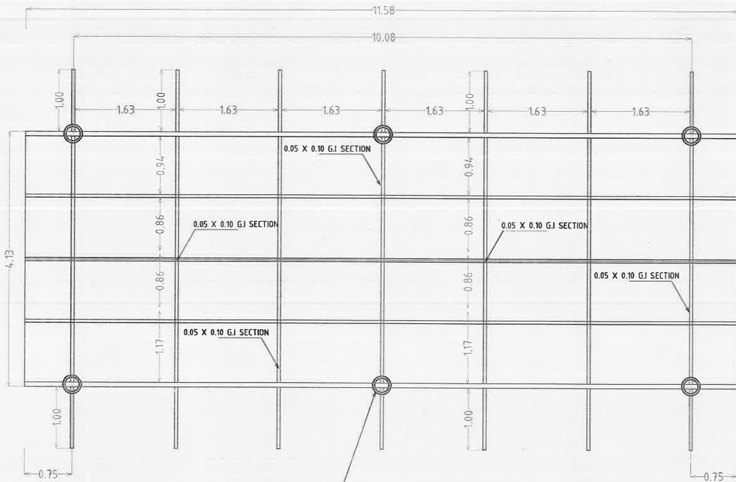
PRECAST RCC PILLAR PLAN
