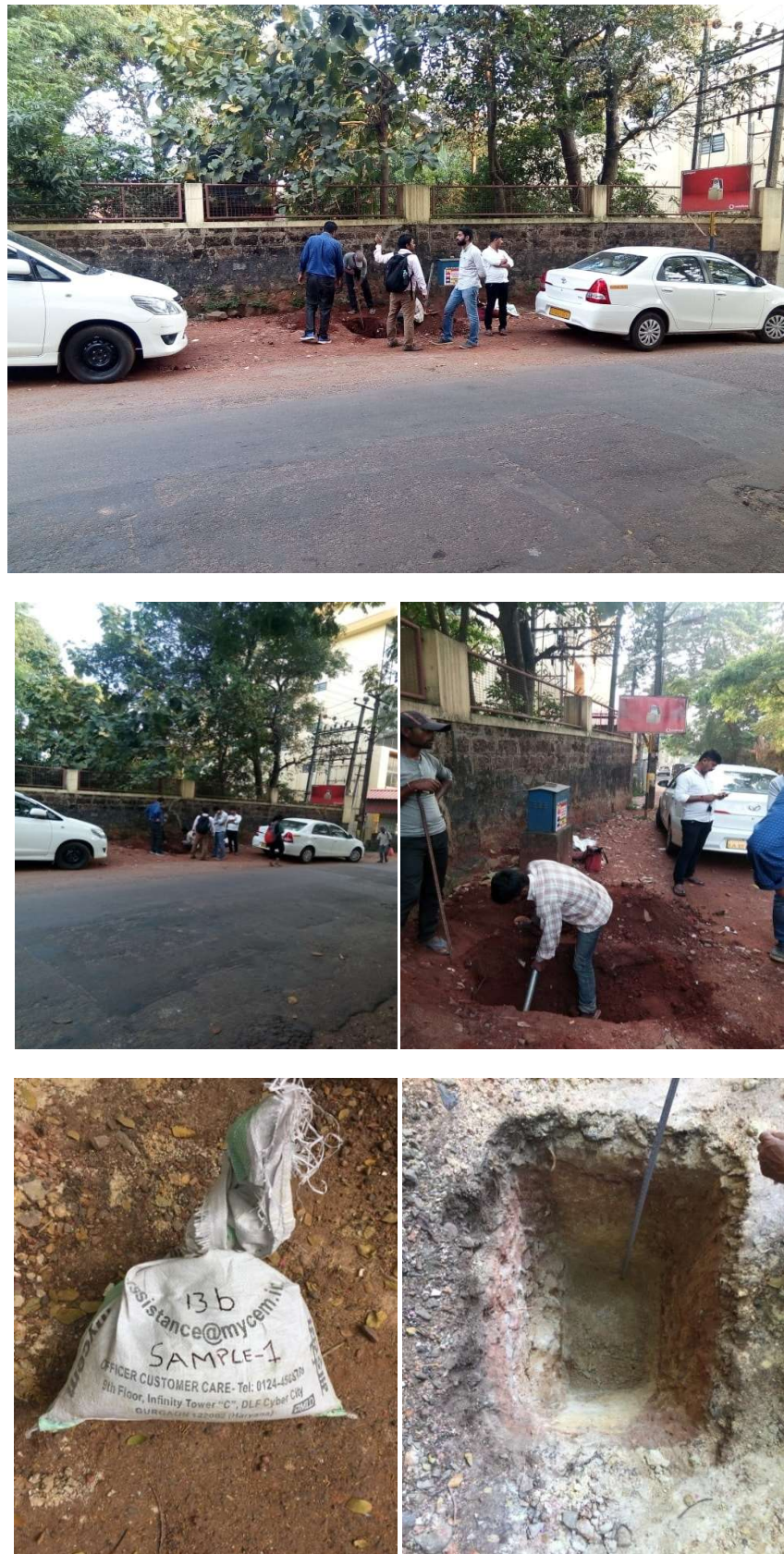
Figure 3-1 Trial Pits Survey Site Photographs
